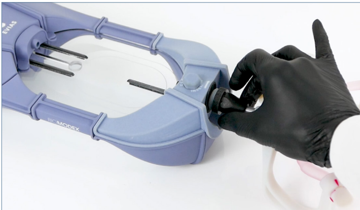
7 / Connect the black Quick Connect of the Station Approach Connector to the black approach plug of the Station.
